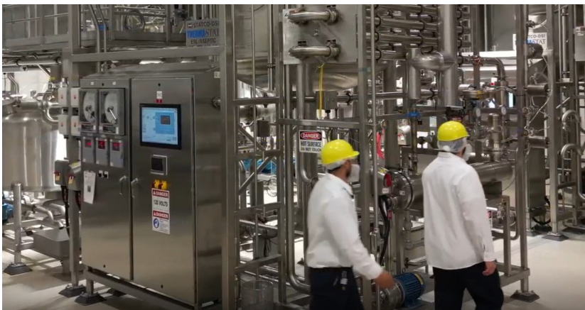
Statco-DSI's combination Therna-Stat UHT processors – capable of producing both ESL and aseptic products in compliance with the PMO and CFR-113, respectively.
